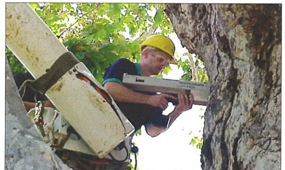
Drilling into a sycamore with a Resistograph.
